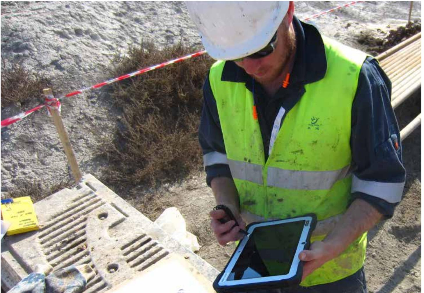
Rotary core sample descriptions and mechanical log data being entered into the pLog software. A stylus is being used in this photograph, but the touch-sensitive screen can be used equally well with bare or gloved hands.
